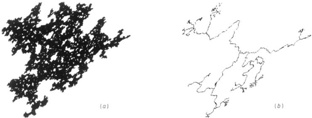
Figure 1. (a) Typical 2D percolation cluster on a triangular lattice, grown to a maximum chemical size of L = 400 . (b) The skeleton of the cluster shown in (a). Note the increasing number of branches as l increases. Although a few small loops are evident, their contribution to the total mass of the skeleton is negligible.
